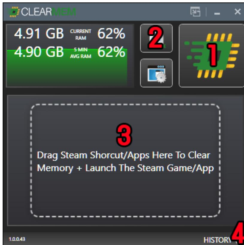
1. **Engage Memory Clearing** – Clicking this button will engage the Memory Clearing and the overlay showing the progress will show up.
